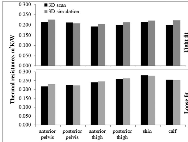
**Figure 2** The thermal resistance of the real and virtual sweatpants for individual body regions.
